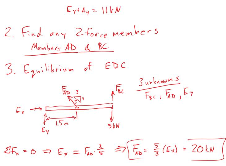
$\begin{aligned} & \xi F_{y=0} \implies E_{y} + F_{AD} \cdot \frac{4}{5} + F_{BC} - 5 kN = 0 \\ & E_{y} + 16 kN + F_{BC} = 5 kN \\ & E_{y} + F_{BC} = -11 kN \end{aligned}$
