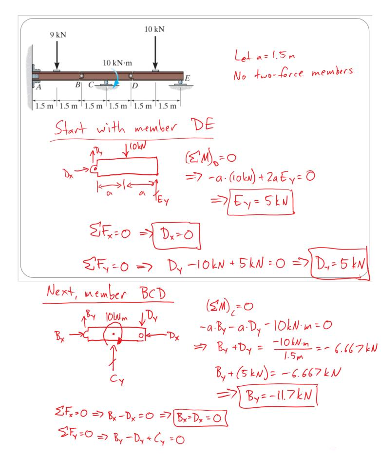
$$\begin{aligned} \sum F_{Y} = 0 \implies B_{Y} - D_{Y} + C_{Y} = 0 \\ (-11.667 kN) - (5kN) + C_{Y} = 0 \implies C_{Y} = 16.7 kN \end{aligned}$$
